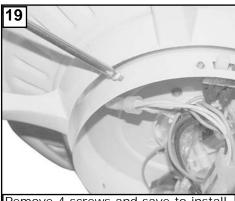
Remove 4 screws and save to install switch housing.
